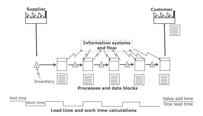
A Value Stream Map is a high-level view of the whole process. It starts at the supplier delivering the raw materials, and ends with the customer receiving the end product, mapping every stage of the process within. The map highlights each stage of the transformation, including the wait time and work time, as well the documenting knowledge transfer within the business. A Value Stream Map gives people the information they need to identify waste in their processes, and make changes to eliminate it.
